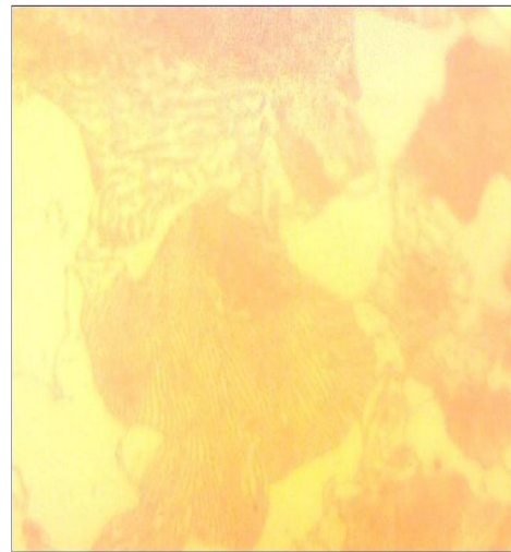
Figure 4- A3-Showing full martensite (dark) when quenched in Ghee Oil
