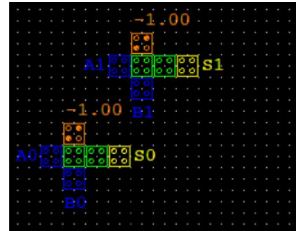
(b) QCA implementation of 2-bit AND
