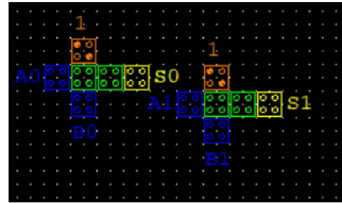
(b) QCA implementation of 2-bit OR
