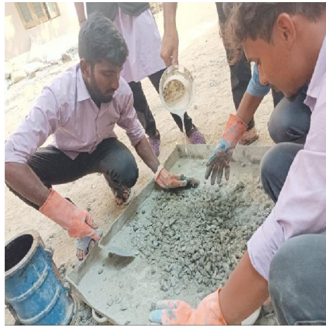
Fig 1: Casting Of moulds
