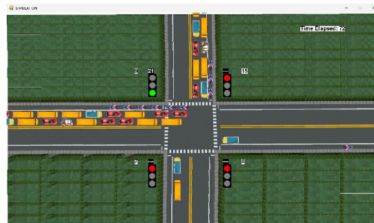
Fig 3.1: Simulation showing signal status, countdown and vehicles crossed
