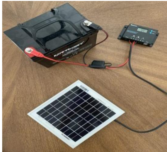
Fig. Block Diagram of Solar Battery Charger
