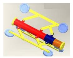
An Underwater Pipeline Inspection Robot Based on Raspberry Pi[2]
