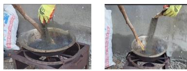
Casting and Molding: The mixture is poured into molds placed on oiled surfaces. Multiple pours and tapping ensure proper compaction and smooth surfaces. Vibration-assisted consolidation further improves block strength and quality.
