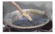
Homogeneous Mixing and Sand Incorporation: The melted plastic is mixed with warm, dry sand and fly ash to create a homogeneous mixture. Mixing is done carefully to ensure even distribution of materials, resulting in strong and visually appealing blocks.
