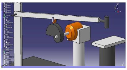
2) To discover torque pressure transmitted we have two instances CASE 1: while Hammer moves downward Given: (BC)=h =153 mm= 0.153 mm Torque =30.55 N-m = 30.55×103 N-mm Length of hammer rod=420mm = 0.42 m Torque pressure = Tmax × length of hammer rod =30.55 ×0.420.153
