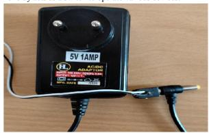
**Figure 7:** 5V 1A power adapter
