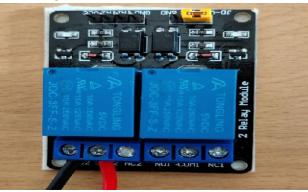
Figure 6: Relay module
